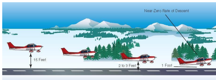
Example of a well-executed round out and proper landing attitude
